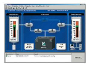
port, and monitor its working status. The UPS comes with Powerware LanSafe™ software, free of charge. This UPS management software gives you control and visibility over all your UPSs, using an intuitive, graphical interface.
