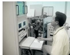
All Comet UPS are manufactured in MCE's Costa Mesa, California flagship plant. Before shipment each unit is individually tested and operated for four to eight hours, ensuring reliable on site operation.
