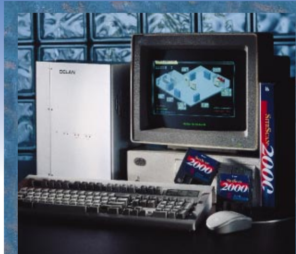
SiteScan centralized monitoring system provides operating status for all computer support systems.
