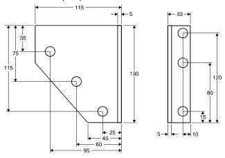
NOTES: All dimensions are in millimeters. All holes are 13 mm (0.51") in diameter. M12 x 30 hardware is provided.
