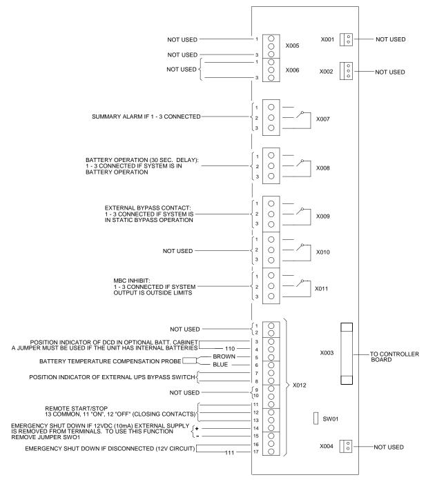
X007-X011 ARE CHANGE OVER RELAY CONTACTS (NOT TO EXCEED NEC ARTICLE 725 C CLASS 2 LIMITS)
