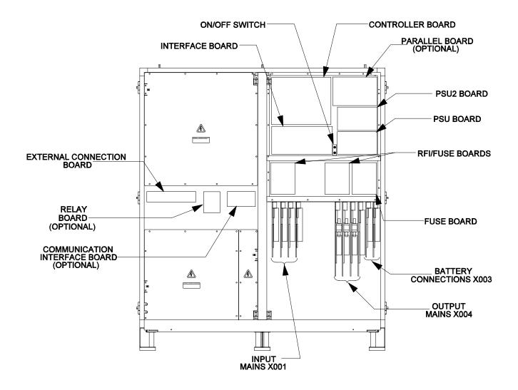
**Figure 3: UPS Wiring Terminations**
