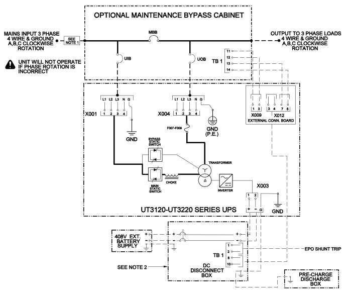
**NOTE 1:** Size the mains input overcurrent protection device per applicable codes. See the table below for mains input voltage and current ratings.
