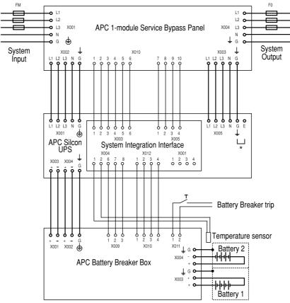
6.1.2 UPS with 1-module SBP and External Battery via Battery Breaker Box - Single Utility - 4-wire Grounded WYE service
