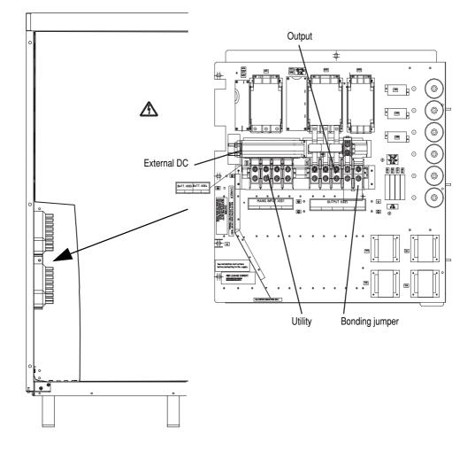
Inside view of left side 15kW-40kW 208V, 30-40kW 480V
