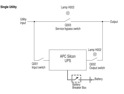
$System \ Integration \ Interface \ (SII) \ is the \ control \ link \ between \ UPS \ and \ system \ main \ switches \ as \ shown \ above. The \ purpose \ of \ the \ SII \ is \ to \ ensure \ correct \ operation \ of \ switches \ without \ losing \ system \ output \ power.$
