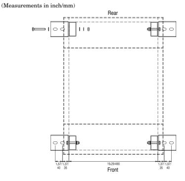
6.4.1.4 Seismic Anchoring 23.62 inch/600 mm Cabinet Mounted outside Frame
