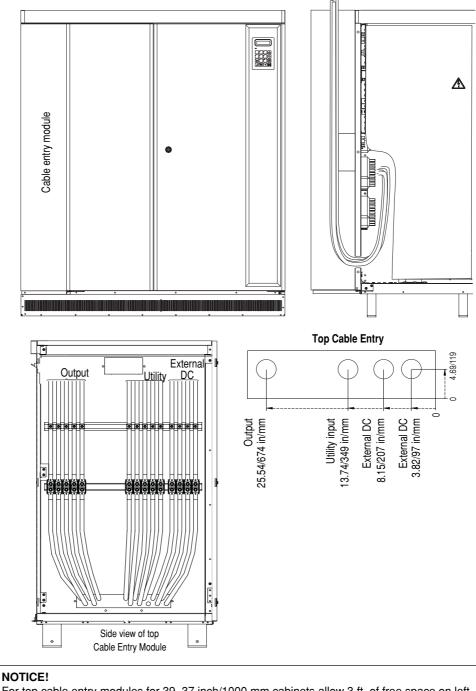
For top cable entry modules for 39. 37 inch/1000 mm cabinets allow 3 ft. of free space on left side for cable connection.
