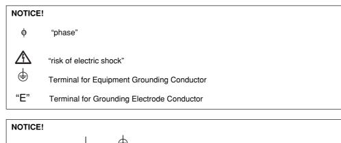
Terminals marked  $\stackrel{\downarrow}{=}$  and  $\stackrel{\textcircled{\oplus}}{=}$  are electrically connected to the terminal marked "E"
