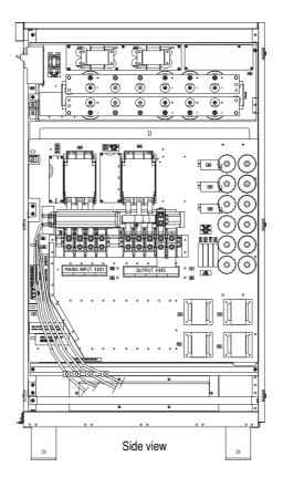
DC cables in Top Entry Module for 39.37 inch/1000 mm Cabinet
