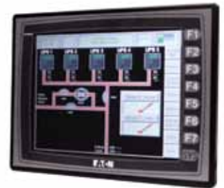
Eaton 10 inch LCD SBM screen
