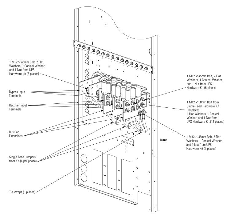
**NOTE** Install bus bar extensions to back side of rectifier input bus bars to provide clearance for bolts and wires.
