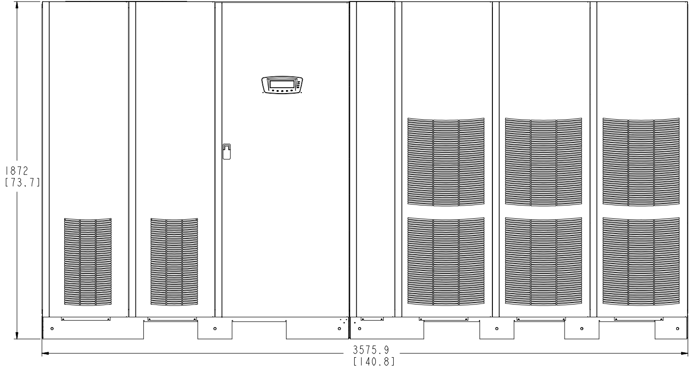
Figure 3-1. UPS Cabinet Dimensions – Three UPM (Front View)
