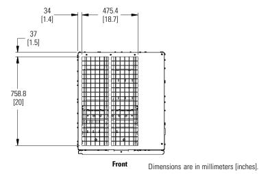
Figure 3-3. FI-UPM Cabinet Dimensions (Top View)
