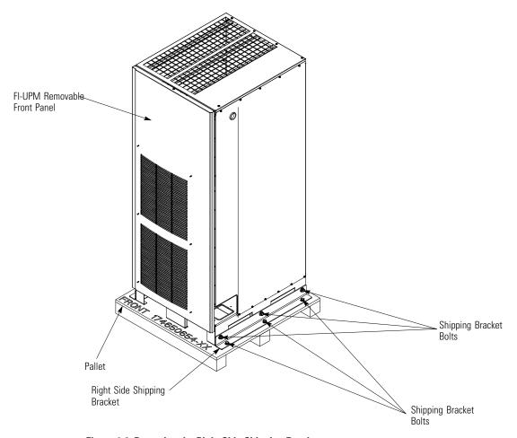
Figure 4-2. Removing the Right Side Shipping Bracket
