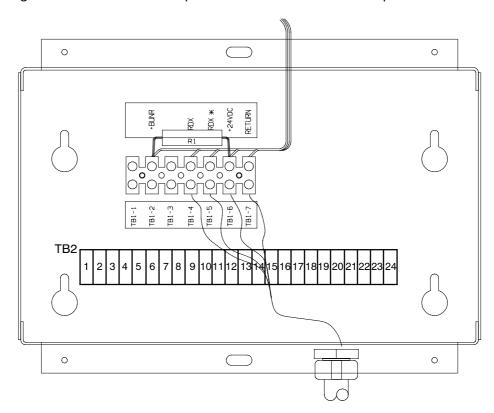
Figure 6-5. Supervisory Contact Module
