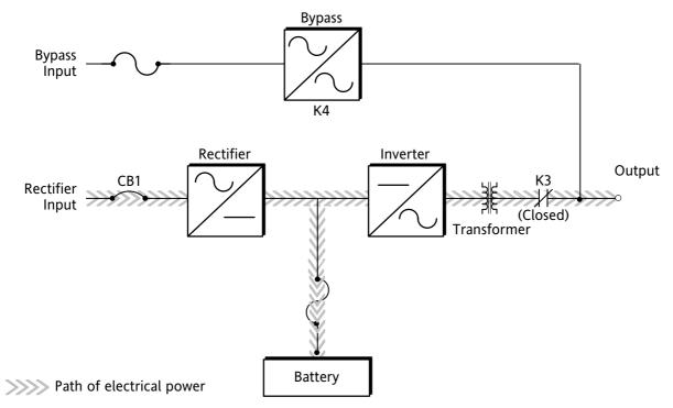
Figure 3-1. Path of Current Through the UPS in Normal Mode
