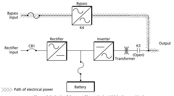
Figure 3-2. Path of Current Through the UPS in Bypass Mode
