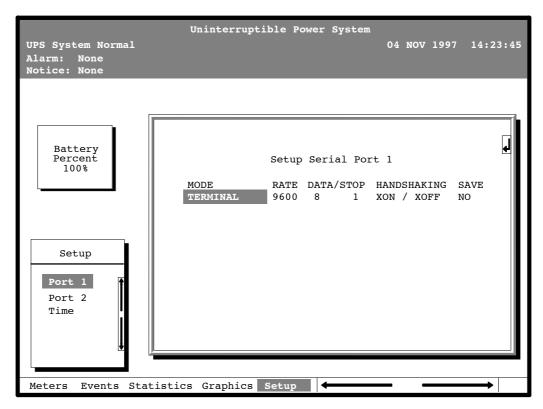
Figure 5-10. Setup Serial Port 1 Screen
