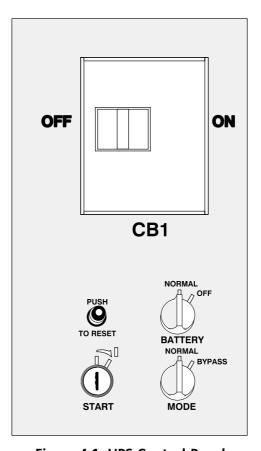
Figure 4-1. UPS Control Panel
