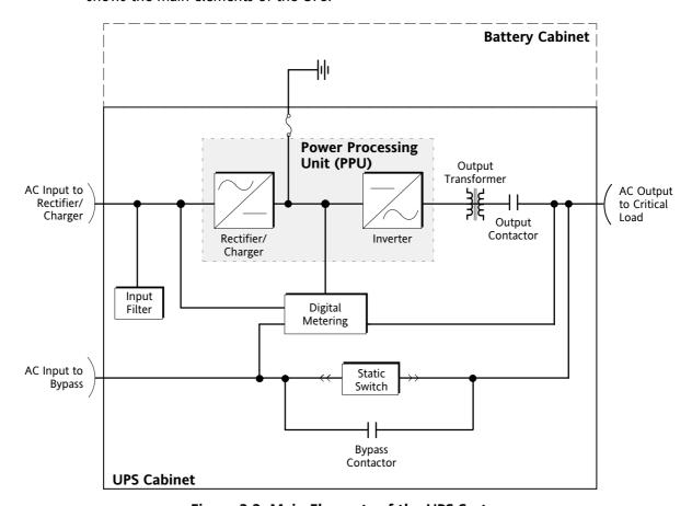
Figure 2-2. Main Elements of the UPS System
