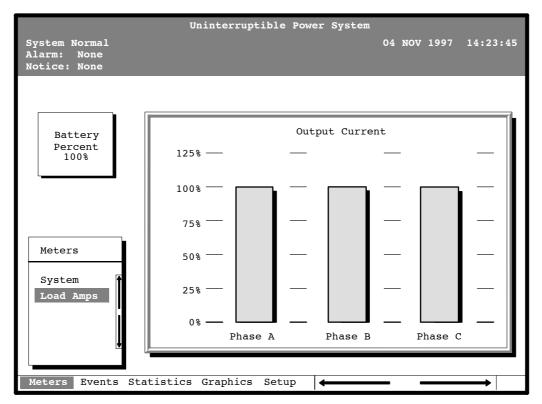
Figure 5-4. Load Amps Meters Screen
