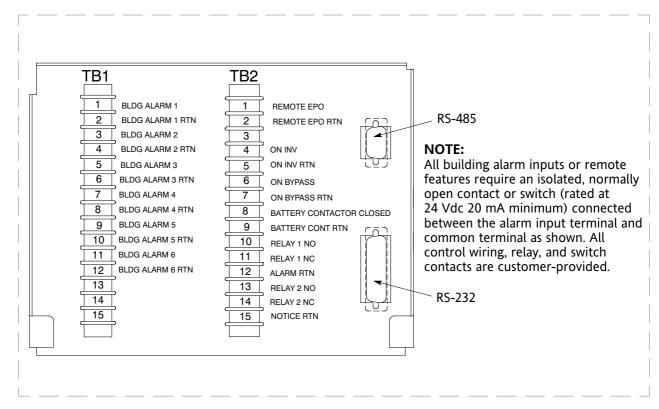
Figure 6-1. External Connections for Building Alarm Monitoring
