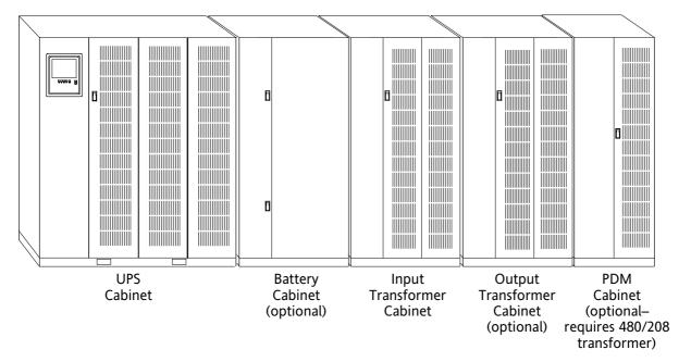
Figure 2-1. Typical Powerware 9315 UPS System
