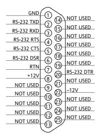
Figure 7-4. Port 2 (DB-25) Pin Assignments
