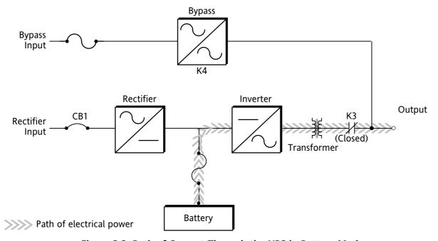
Figure 3-3. Path of Current Through the UPS in Battery Mode
