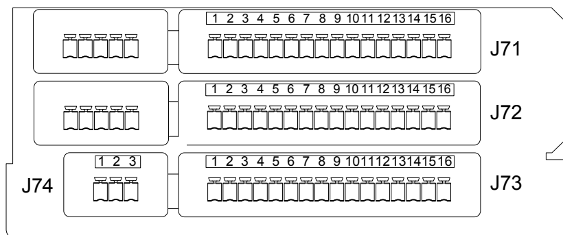
Figure 48 Control wiring, Programmable Relay Board
