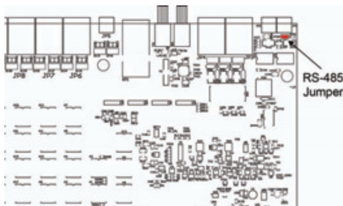
Figure 21 SM-BRC RS-485 Jumper Locations
