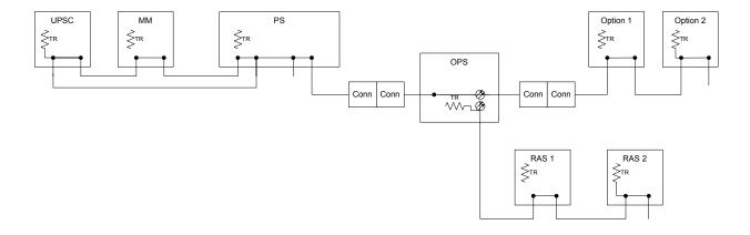
**Figure 7** shows two additional options connected to the CANbus. These options could be an OCDO or an OCDI option. When these options are installed, the termination is enabled on the last unit on the CANbus.
