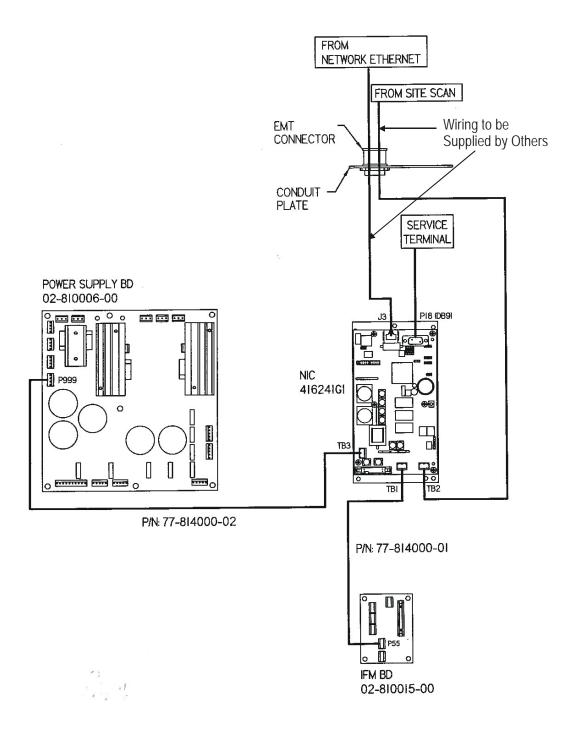
Liebert Global Services can attach a service terminal at P18 (DB9) on the top right side of the board.
