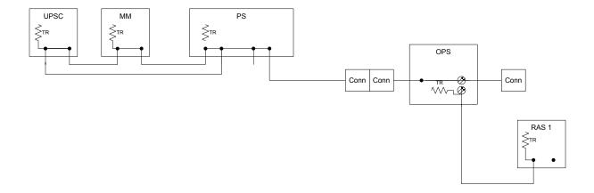
In **Figure 5** an Option Power Supply (OPS) and a Remote Status Panel (RAS) have been added to the CANbus. The Option Power Supply contains an isolated CANbus repeater so the CANbus in the OPS/RAS loop is considered to have originated at that point only to the RAS panel. The isolated output of the OPS is pre-configured with a terminator on the included terminal block.
