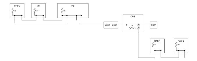
**Figure 6** shows an additional RAS panel and the termination jumper moved from RAS #1 to RAS #2. This is accomplished by removing the termination jumper from RAS #1 and installing the jumper in RAS #2.
