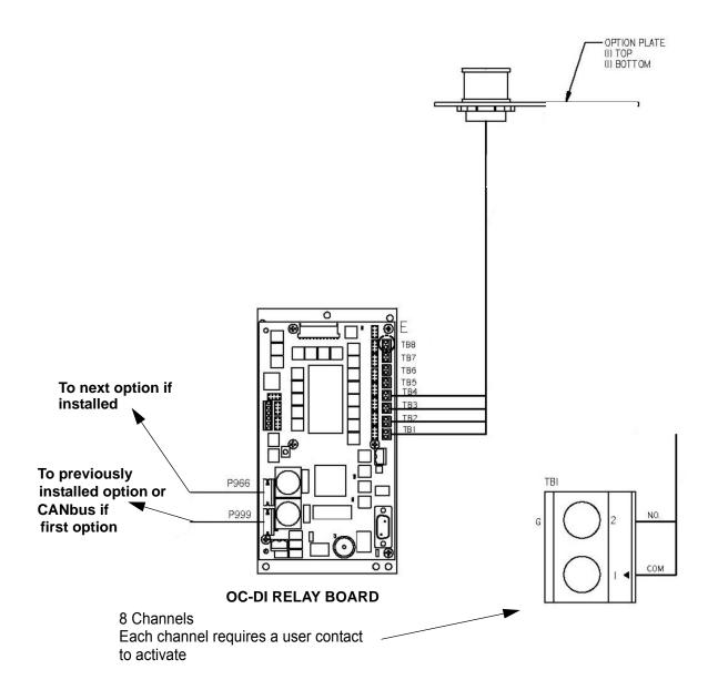
All harnesses and cables should be dressed and secured via tie wraps to make sure they do not move when the option door is closed. Excess cabling should be neatly coiled and tie wrapped
