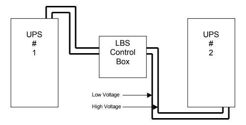
Figure 82 LBS Assembly Diagram
