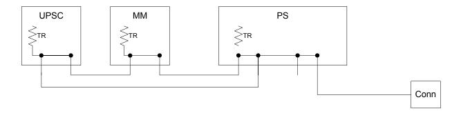
In **Figure 4** the CANbus is terminated on the UPS Control Board that connects to the MicroMonitor (MM) board and to the Power Supply. The Power Supply provides an electrical connection point for the CANbus in addition to power for the CANbus. It does not actively connect to it. The final CANbus termination is on the Micro Monitor board.
