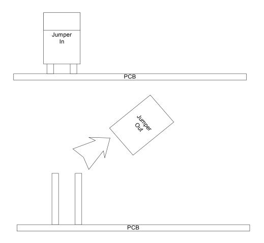
**Figure 9** shows an example of jumper removal. Please consult the documentation with each option to determine the location of the termination resistor jumper.
