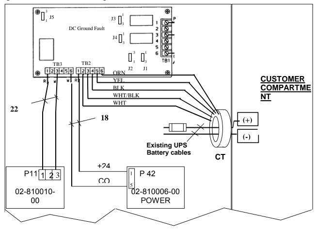
5. Configure the program jumpers on the DC Ground Fault Detector as follows:
