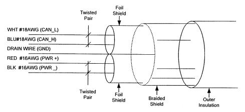
Note: Connection to Drain Wire automatically connects Braided Shield and Foil Shield
