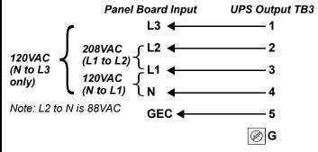
**CAUTION:** It is important for the installing electrician to clearly identify the connections for future reference. Refer to NEC 215-8 and 210-4(d).
